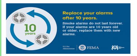
Each smoke detector should be replaced 10 years after the date of installation. If you're not sure when it was installed, check the back of the smoke detector for the manufacture date and add 10 years to it to get the expiration or replacement date. Most CO alarms expire after 7 years, so if you have a combo smoke and CO detector, you should replace it every 7 years.
